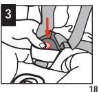
Press red button on buckle to release the buckle plates. Place harness over sides of child restraint. Remove child.
